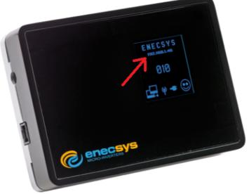
On the display, just below the word 'Enecsys' is the Gateway IP Address. This is the local address of your gateway. Open a web browser and type in the IP address from your gateway.
