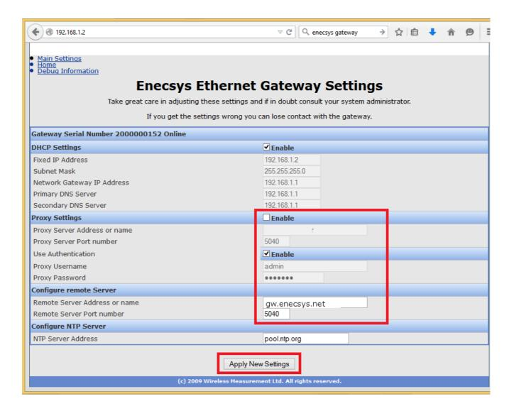
Change the 'Remote Server Address or name' from the old Enecsys Monitoring server **gw.enecsys.net** and click 'Apply New Settings'. The gateway will reboot and in a f minutes, the little face on your gateway should be smiling again.
